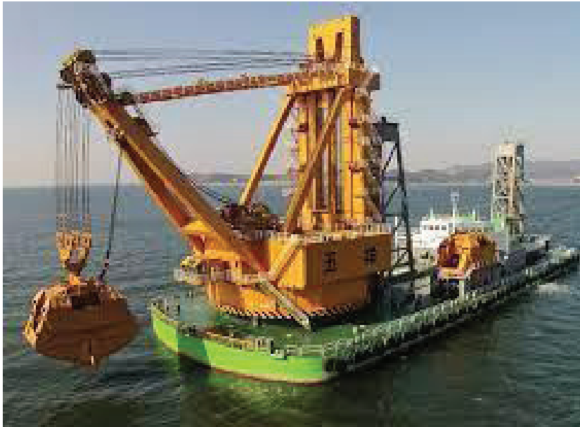
Figure 3. Seabed quarrying vessels: grab and bucket dredger (top); trailing suction hopper dredgers
